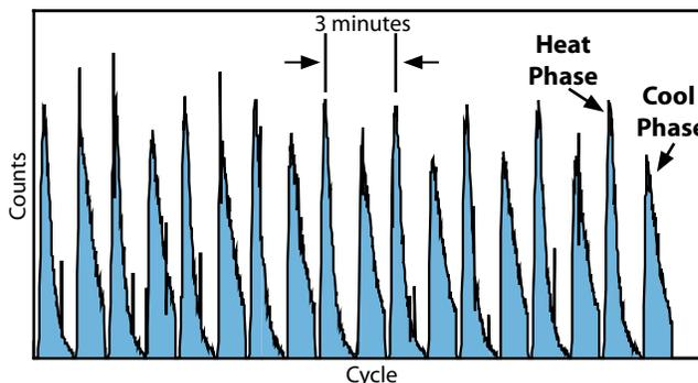
Figure 4 is a typical COOL-X output flux vs Time. Specific units may have more counts during the heating or cooling phase, or all of the counts in one of the two phases.
