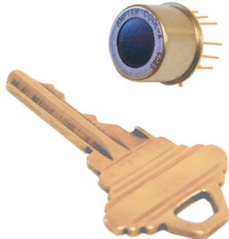
The COOL-X is a novel, miniature X-ray generator which uses a pyroelectric crystal to generate energetic electrons that produce X-rays in the target material (Cu). The hermetically sealed package has a thin beryllium window which allows the X-rays to be transmitted. The COOL-X does not use radioisotopes or high power X-ray tubes. It is a self contained, solid state system which generates X-rays when the crystal is thermally cycled.
