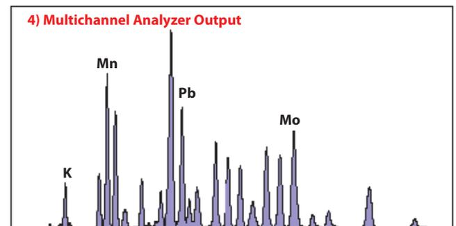
Trace 1 above shows the input to the DP5, which is the output from a reset-type charge sensitive preamplifier. This is processed by the analog prefilter producing the prefilter output shown in Trace 2. This is digitized and then processed digitally, producing the DP5's shaped output shown in Trace 3. Finally, the DP5 creates a multichannel analyzer (MCA) type output spectrum shown in Graph 4.
