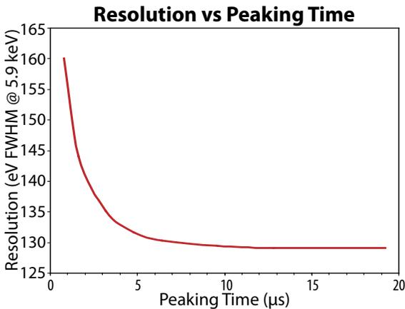
Figure 4. Resolution vs. Peaking Time for the SDD.
