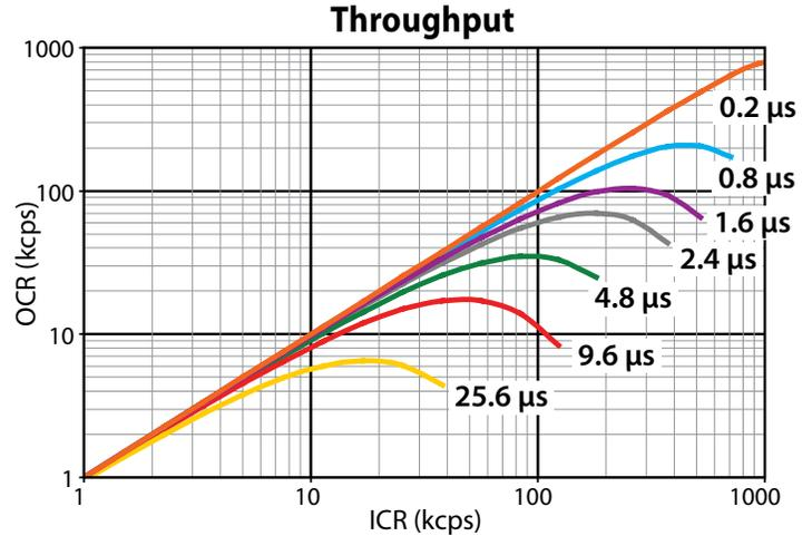
Figure 3. Throughput with the SDD. Due to the detector's smaller capacitance, a much shorter peaking time is used in the shaping amplifier without sacrificing resolution. Typically  $9.6\text{ }\mu\text{s}$  or less is used. This dramatically increases the throughput of the system.
